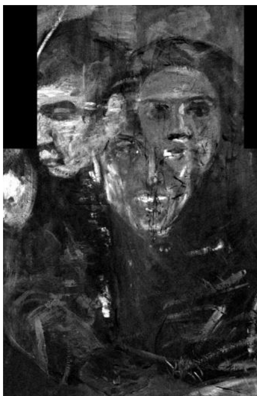
Figure 4 MA-XRF elemental map for mercury (Hg) showing a hidden face. (Image: University of Antwerp/Geert van der Snickt.)
